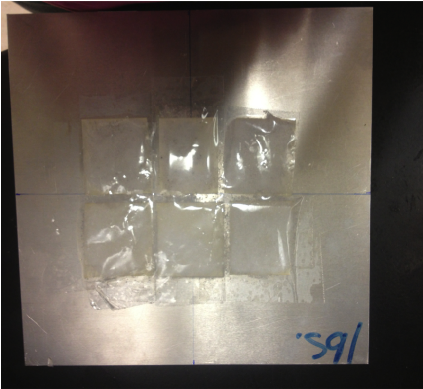
Figure 2.14: Powdered samples arranged on a aluminum plate for exposure and imaging
